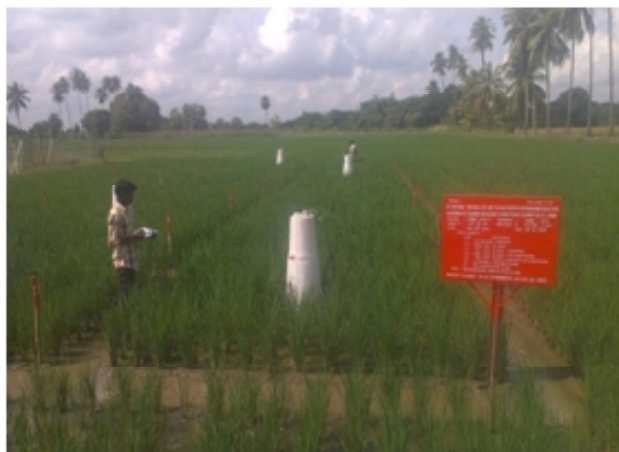
Fig. 2. Methane gas extraction from the field by base chamber method.
